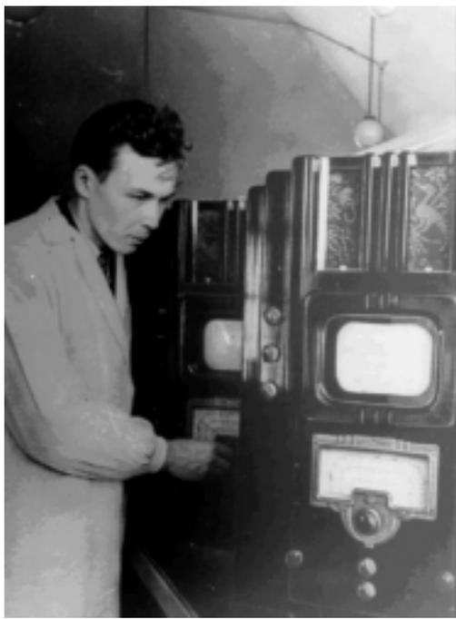
A. Raspletin's laboratory worker A. Klopov prepares 17TN-1 TV sets to formal acceptance on "Radist" factory
